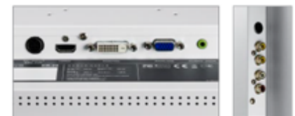
Analogue, DVI, S-Video, CVBS and HDMI inputs for video device or PC data feeds
